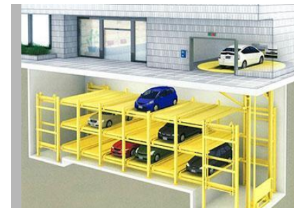
Horizontal Circulation Parking System
